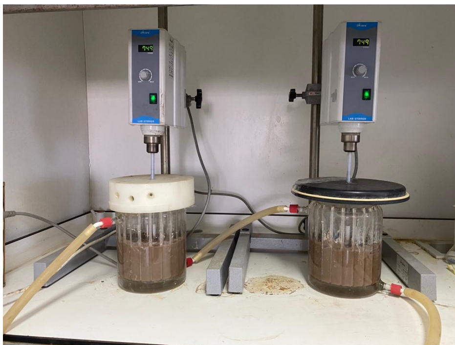
Figure 3.19 Leaching Tests Experimental Setup
