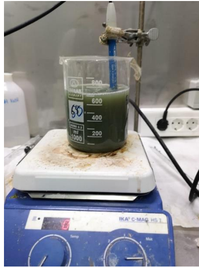
Figure 3.23 Neutralization - Selective Precipitation Tests Experimental Setup
